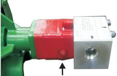
HYDRAULIC MOTOR SPEED/ WATER FLOW MAY BE SLOWED BY OPENING (TURN CCW) NEEDLE BYPASS VALVE. INITIAL SETTING TO BE BACKED OUT 1/4 TURN FROM CLOSED. TO PURCHASE INDIVIDUAL PARTS ON THIS PAGE PLEASE SPECIFY THAT THEY ARE FOR A KE-FCSPWP WATER PUMP
